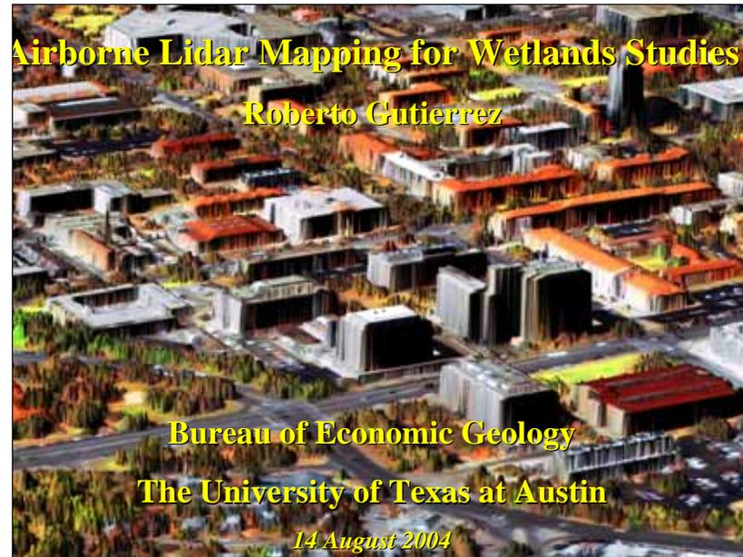
A 1m x 1m resolution digital elevation model of the University of Texas campus computed from airborne lidar. Draped over the lidar DEM is a 1m resolution IKONOS satellite image.
